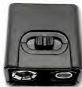
TOGGLE SWITCH ON/OFF: 2 OR 6 LEDS ON/ OFF
